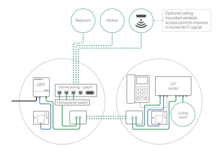
Further to the second option, this setup cables back from the CP router position within the property to the under stairs/service cupboard position of the Openreach ONT for the location of a patch panel. This means that, as much as possible, any structured cabling is discreetly located out of sight.
