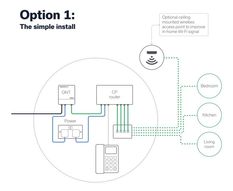
The simplest installation involves the provision of the Openreach equipment (i.e. the ONT will be positioned adjacent to the outside wall) to which the customer then attaches the router, provided by their communications provider (CP).
